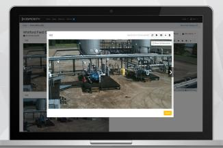
Osperity initially deployed the solution to a select number of high priority well sites. Users were able to view on-demand live images of the pumpjack stuffing box area and rod for all sites, and live video to show rod cadence.
