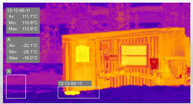
Small leak detected, triggering an alert.
